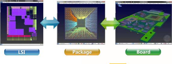
A multi-technology / multi-object environment which shows systems and modules having a complex hierarchical structure, similar to LSI/PKG/PCB, as a single unit is a powerful tool for considering total optimization trade-offs.
