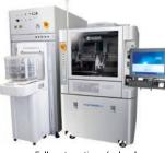
Fully automatic wafer level dispensing machine
