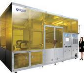
Fully automatic sealant dispensing system for FPD production
